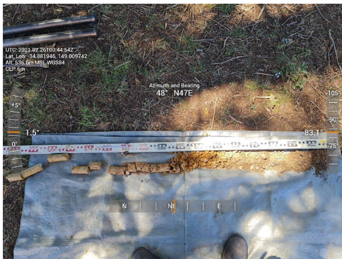
Figure 12: Soil Profile 2 – Effluent dispersal area
